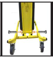
**Step 4:** From the back of base, slide Release Mechanism, (left to right) through channel aligning center threads with center of channel.
