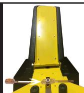
Step 4: Turning clockwise, screw gas spring into release mechanism turning 12 full rotations.
